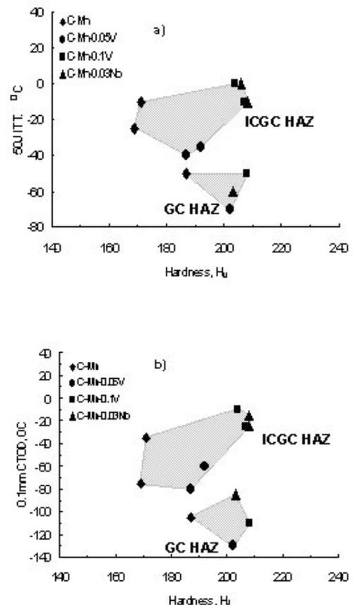
Figure 11 Effects of hardness and vanadium (and Nb) on a) the 50J ITT and b) the 0.1mm CTOD transition temperature of simulated welds, inter-critically reheated to 750 $^{\circ}$ C and 800 $^{\circ}$ C.
