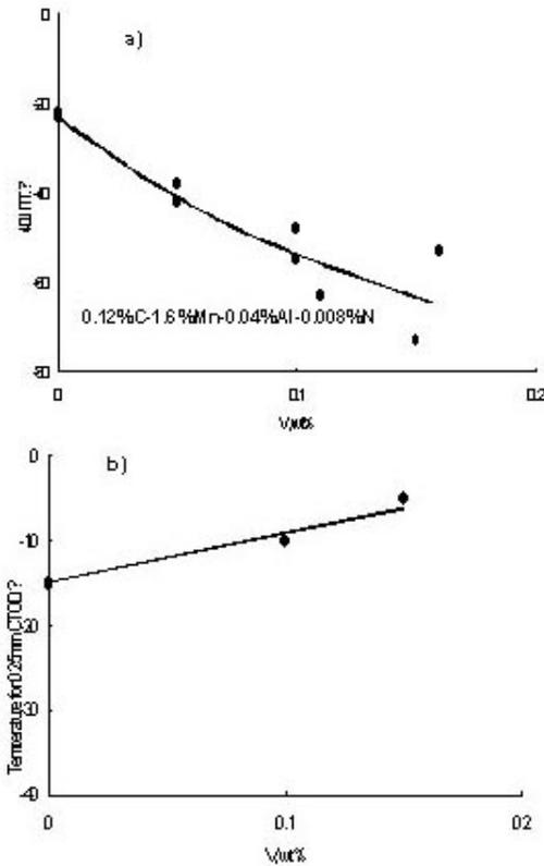
**Figure 9** The effect of vanadium on a) the 40J ITT and b) the 0.25mm CTOD transition temperature, at constant CEV= 0.38, in multi-pass welds welded at 2kJ/mm ( $t_{800/500} = 12$  secs), as-welded. N.B. The CTOD transition temperature was a lower bound value.
