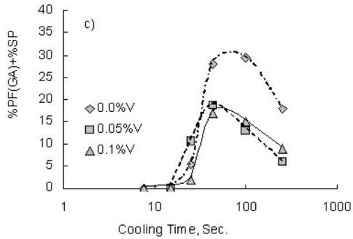
**Figure 2** The effect of weld cooling time on the amount of a) grain boundary polygonal ferrite. b) ferrite with aligned second phase c) grain boundary allotriomorphic + sideplate ferrite, in simulated welds.
