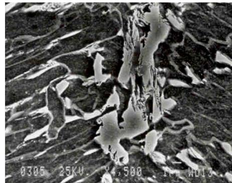
**Figure 6** M-A phase from an inter-critically reheated HAZ.
