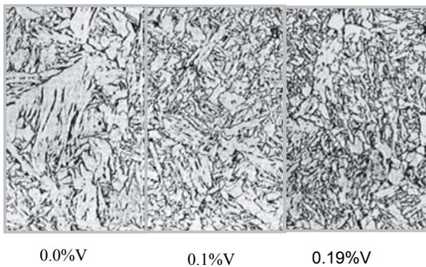
**Figure 3** Effect of vanadium on intra-granular ferrite formation.
