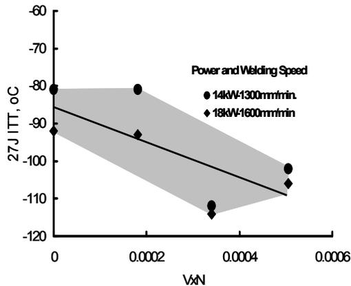
Figure 12 Effect of vanadium on the 27J ITT of CO<sub>2</sub> laser welds
