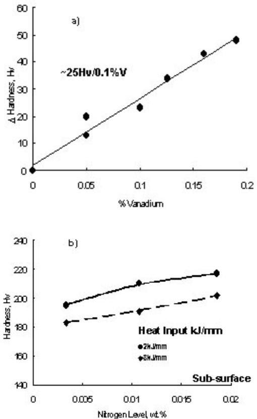
Figure 8 Effects of a) vanadium and b) nitrogen and heat input on the hardness of multi-pass welds.
