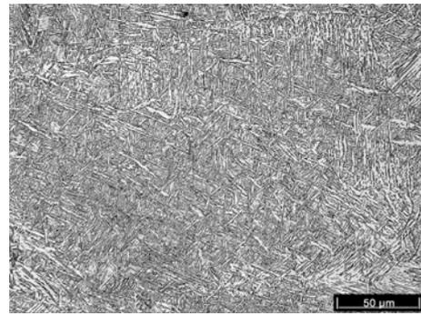
**Figure 5** Intra-granular acicular ferrite in a laser weld.
